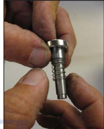
Pull the old spring of the pin and put the new spring on, turn the spring, it fits in a track on the pin
