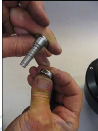
Move pin to the new magnet Important: the magnets should be polarized as before
